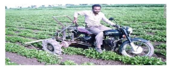
The Bullet Santi, as it is called, has several advantages over other types of cultivators. First, though price estimates vary, it is more affordable than larger tractors. Second, because of its smaller size and lighter weight, the Bullet Santi causes less soil compaction than larger models. Third, the Bullet Santi is fuel efficient—it can plow two acres on just one liter of diesel.
